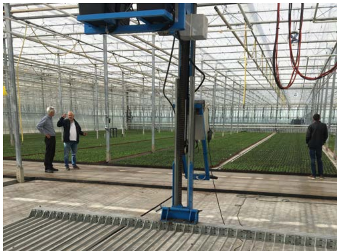
Figure 2. The powered fork system employed at Zuidbaak Nursery for plant movement to and from production beds
