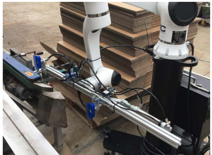
Figure 5. Box-making robotic arm at Baas Nursery
