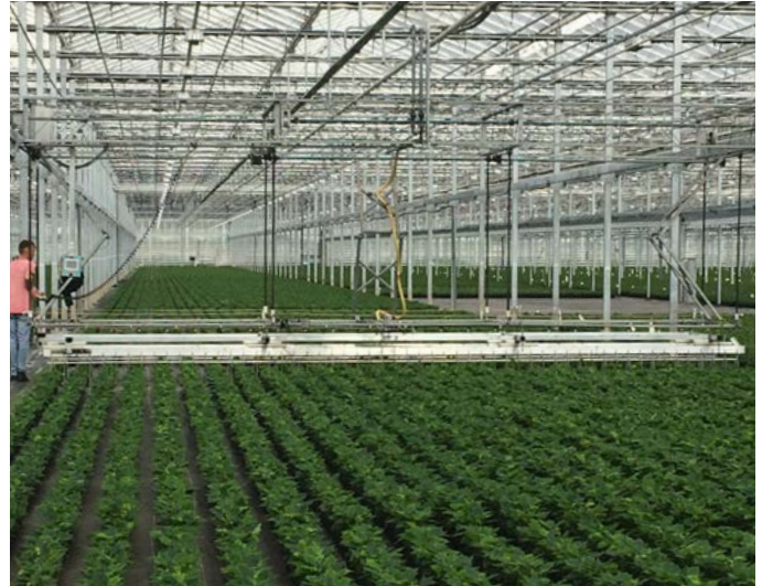
Figure 3. Bed-wide spacing machine employed at Wouters Nursery
