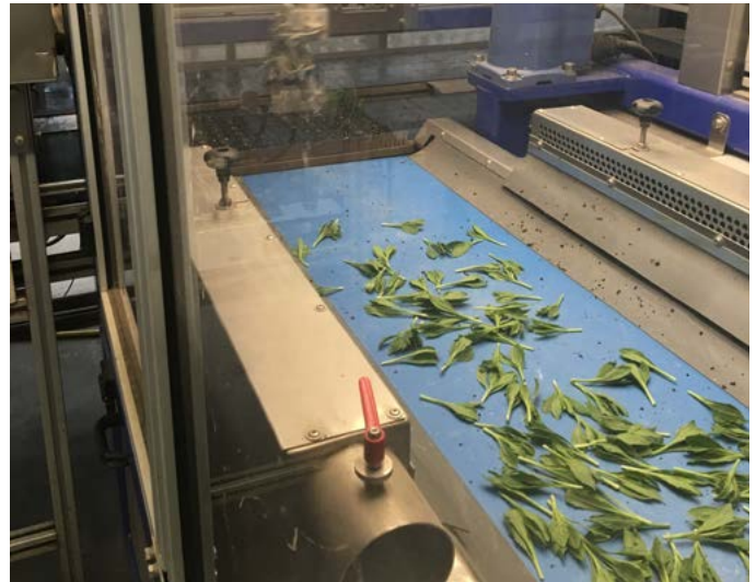
Figure 4. The ISO Group sticking machine in action, handling Osteospermum cuttings at Beekenkamp
